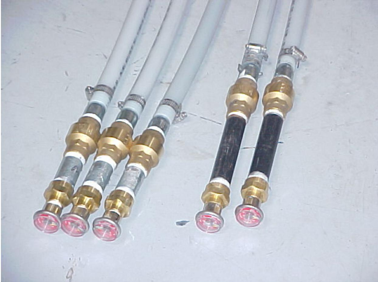
Figure 9. Close-up of Pyroflex check valves and pressure gauges
