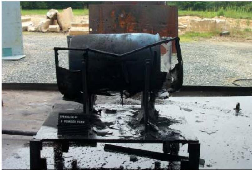
Figure 6. Successful ballistic test with Black Widow/Monnex FIRE Panel variant
