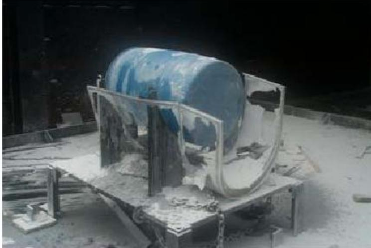
**Figure 5. Post experiment photograph of 3 in. thick powder panel**
