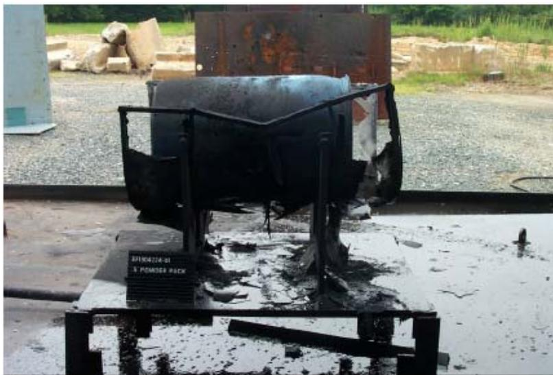
**Figure 9. Post experiment photograph of 0.5 in. powder panel filled with Black Widow**
