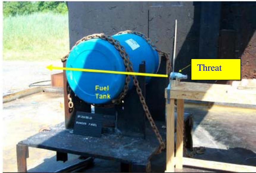
**Figure 1. Experimental arrangement for baseline fire evaluation**
