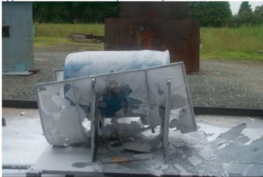
**Figure 7. Post experiment photograph of 1.5 in. powder panel**
