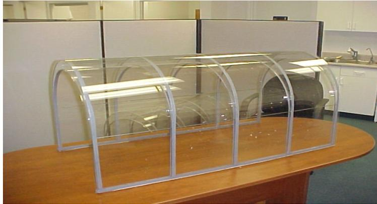
**Figure 2. Prototype powder panel (empty of powder)**
