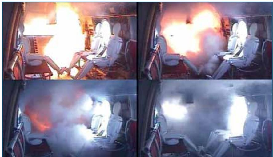
**Figure 3** JLF Firetrace Testing for Rotorcraft Main Cabin Fire Protection
