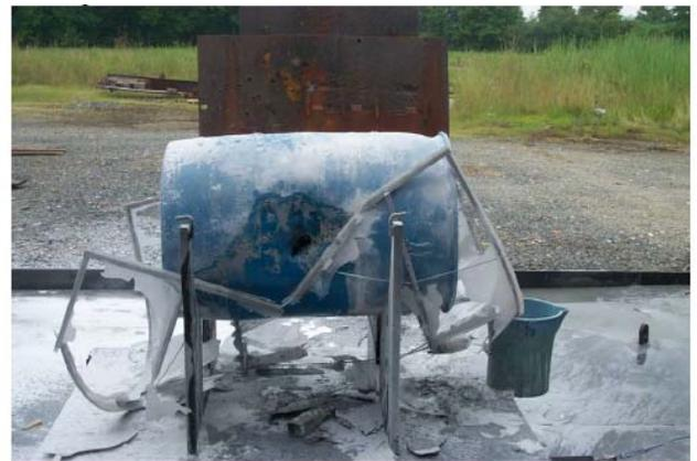
**Fig. 18. Intact fuel tank and shattered powder panel after successful fire protection test.**
