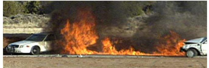
**Fig.10. CVPI burning immediately after impact in baseline test.**
