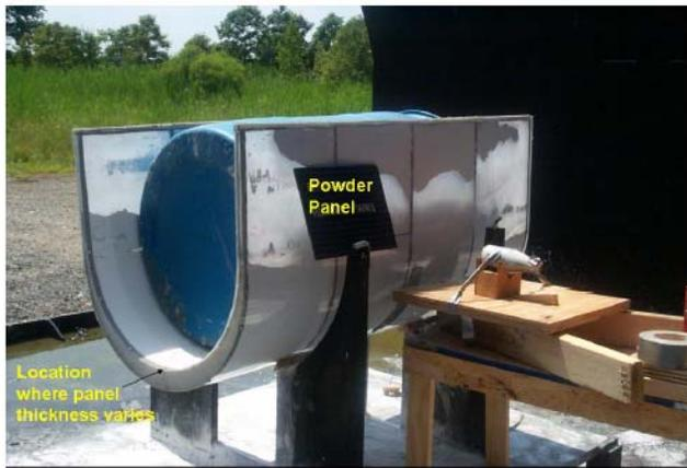
**Fig. 16. Experimental arrangement for baseline fire evaluation.**
