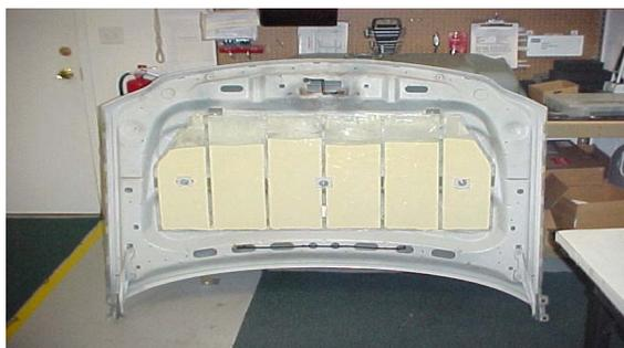
**Fig. 20. Prototype powder panel hood liner unit, mounted in the truck hood.**
