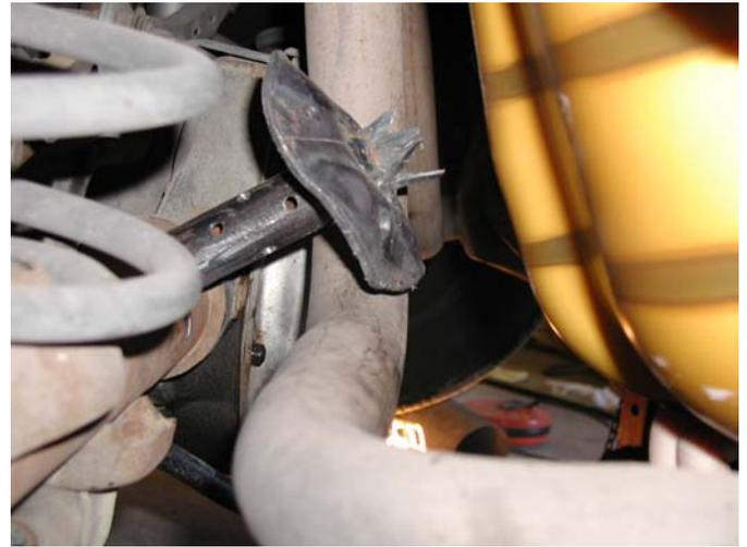
**Fig.7. Fuel tank puncture device in place.**
