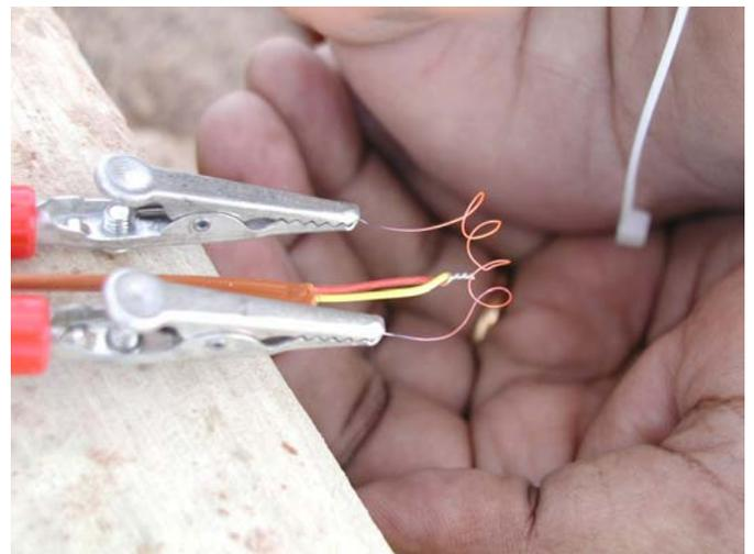
**Fig.8. Ni-chrome wire filament/wire ignition source**
