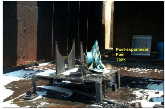
**Fig. 17. Post experiment photograph of unprotected fuel tank damage due to sustained fire.**
