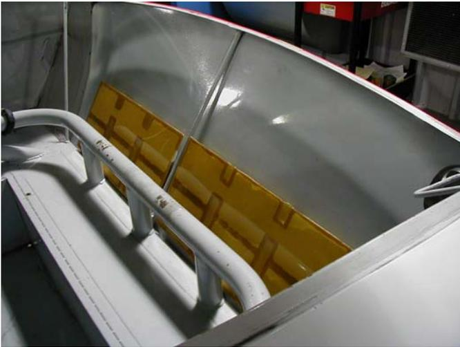
**Fig. 26. Racing powder panel in Nextel Cup car.**
