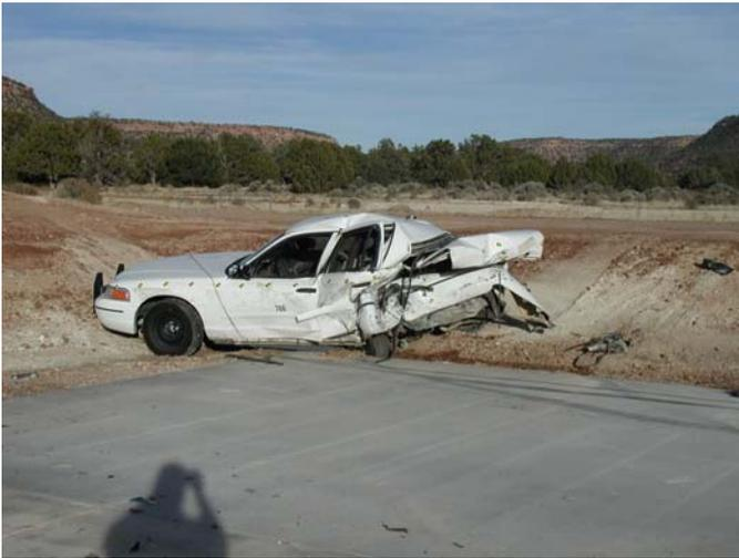
**Fig. 13. CVPI after impact (with panel installed).**
