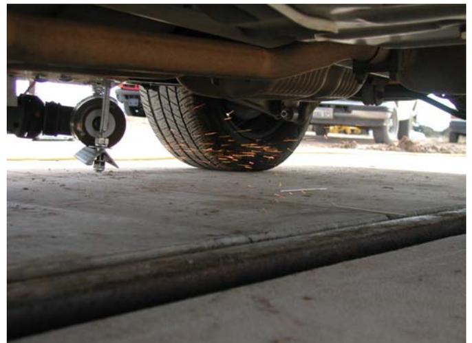
**Fig.9. Spark generating assembly with grinding wheel mounted on the CVPI.**
